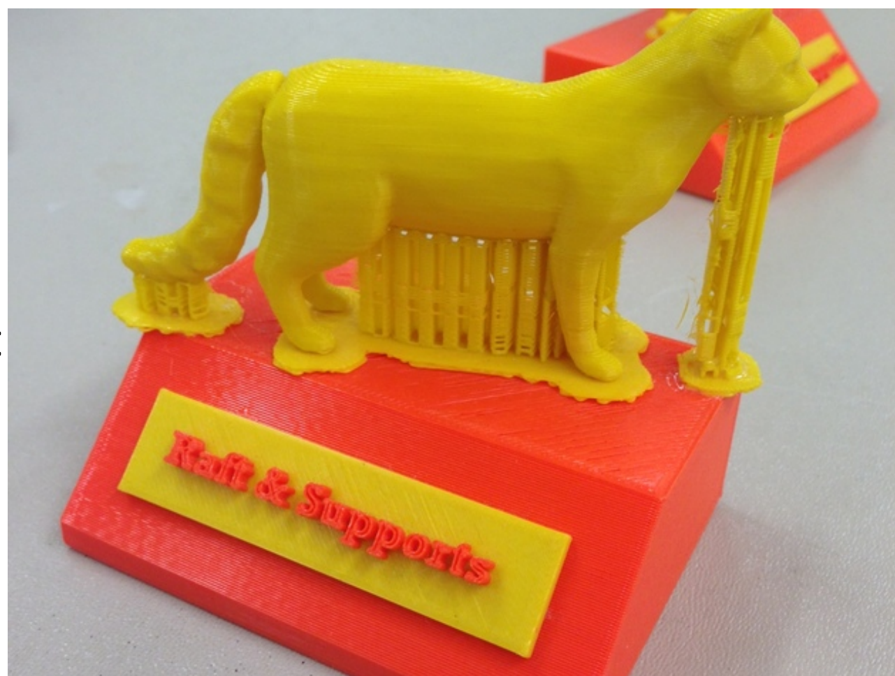
Example of an object with both Rafts & Supports used for stability. Rafts and supports are later removed from the print.
